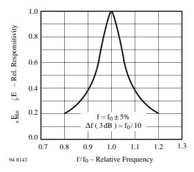
Figure 1. Frequency Dependence of Responsivity
