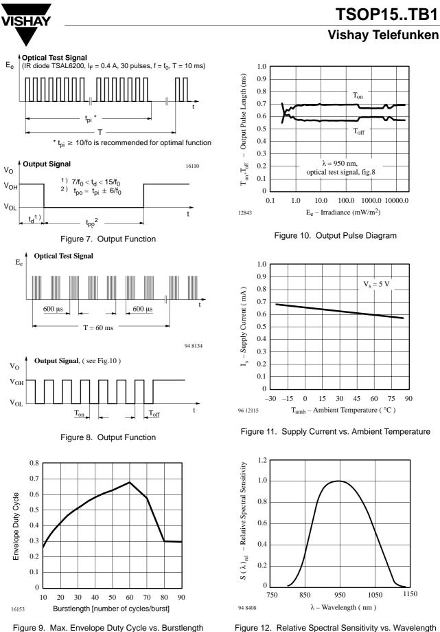
Figure 12. Relative Spectral Sensitivity vs. Wavelength
