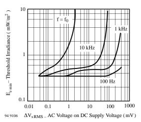
Figure 5. Sensitivity vs. Supply Voltage Disturbances
