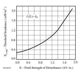
Figure 4. Sensitivity vs. Electric Field Disturbances
