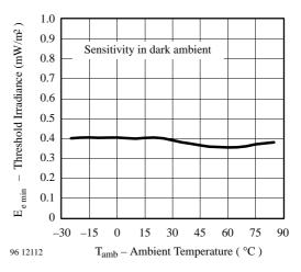
Figure 6. Sensitivity vs. Ambient Temperature
