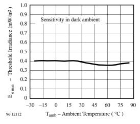
Figure 6. Sensitivity vs. Ambient Temperature
