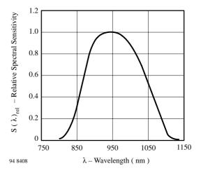
Figure 12. Relative Spectral Sensitivity vs. Wavelength
