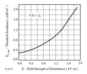
Figure 4. Sensitivity vs. Electric Field Disturbances
