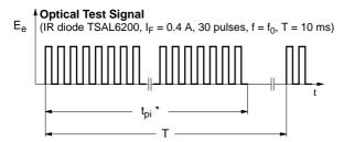
\*  $t_{pi} \ge 10$ /fo is recommended for optimal function
