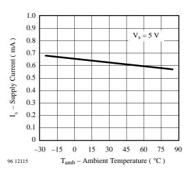
Figure 11. Supply Current vs. Ambient Temperature
