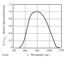
Figure 11. Relative Spectral Sensitivity vs. Wavelength
