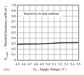
Figure 5. Sensitivity vs. Supply Voltage
