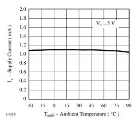
Figure 8. Supply Current vs. Ambient Temperature
