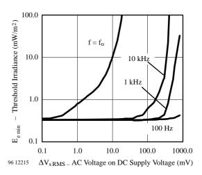
Figure 4. Sensitivity vs. Supply Voltage Disturbances
