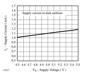
Figure 10. Supply Current vs. Supply Voltage
