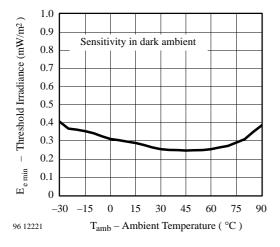
Figure 9. Sensitivity vs. Ambient Temperature
