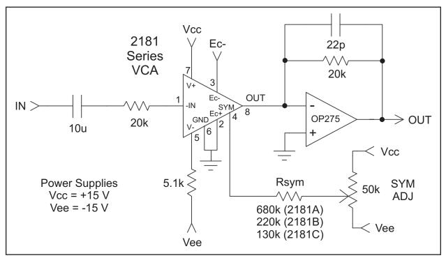
Figure 2. Typical Application Circuit
