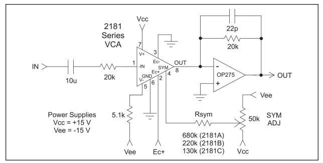
Figure 15. Positive Control Port Using Pin 4
