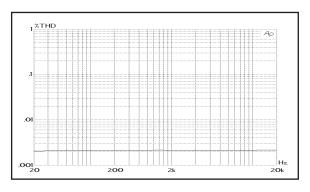
Figure 13. 2181A THD+N vs. Frequency, 0 dB Gain, 1 V
