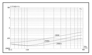
Figure 10. 1 kHz THD+Noise Vs. Input Level, 0 dB Gain
