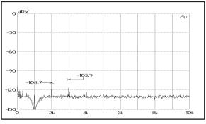
Figure 14. FFT of THD, Typical 2181A, 0dB Gain, 1V, 1kHz
