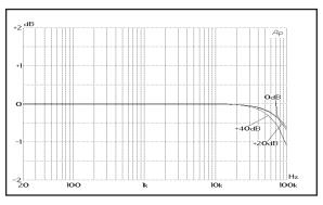
Figure 3. 2181 Series Frequency Response Vs. Gain
