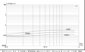
Figure 11. 1 kHz THD+Noise Vs. Input Level, +15 dB Gain
