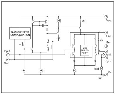
Figure 1. 2181 Series Equivalent Circuit Diagram
