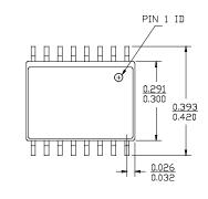
DIMENSIONS IN INCHES  $\frac{\text{MIN.}}{\text{MAX.}}$  LEAD COPLANARITY 0.004 MAX.
