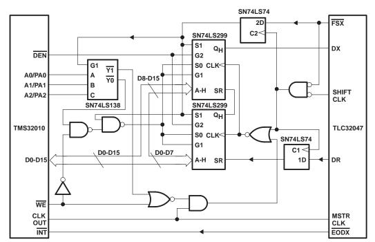
Figure 4-6. TMS32010/TMS320C15-TLC32047 Interface Circuit
