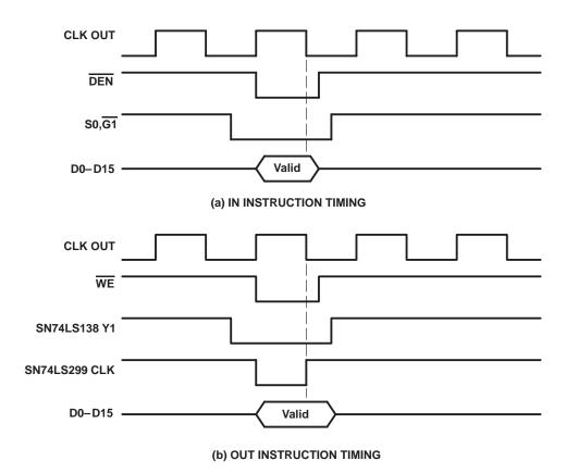
Figure 4–7. TMS32010/TMS320C15-TLC32047 Interface Timing
