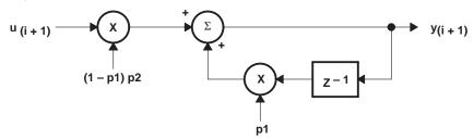
Figure 2-8. First-Order Correction Filter
