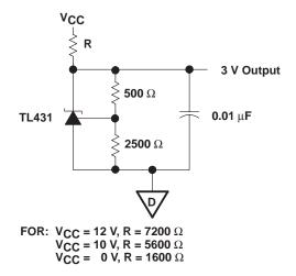
Figure 6-2. External Reference Circuit for TLC32047
