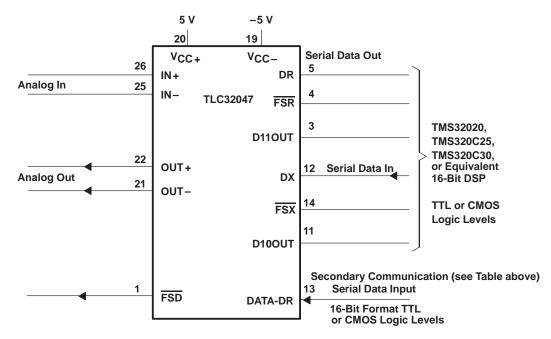
Figure 1-1. Dual-Word (Telephone Interface) Mode
