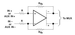
$R_{fb} = R \text{ for } D6 = 1 \text{ and } D7 = 1$ D6 = 0 and D7 = 0 $R_{fb} = 2R$  for D6 = 1 and D7 = 0  $R_{fb} = 4R$  for D6 = 0, and D7 = 1
