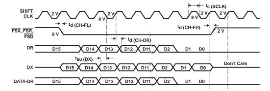
Figure 4-2. Dual-Word (Telephone Interface) Mode Timing
