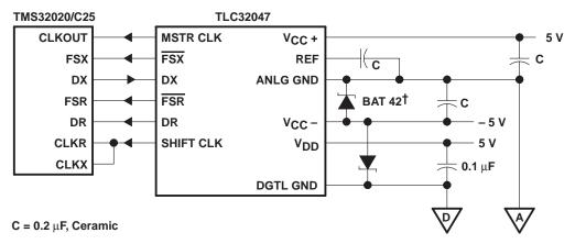
Figure 6–1. AIC Interface to the TMS32020/C25 Showing Decoupling Capacitors and Schottky Diode<sup>†</sup>
