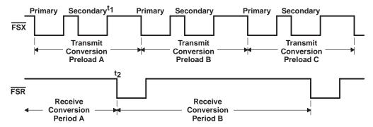
Figure 2–7. More Than One Set of Primary and Secondary DX Serial Communications
