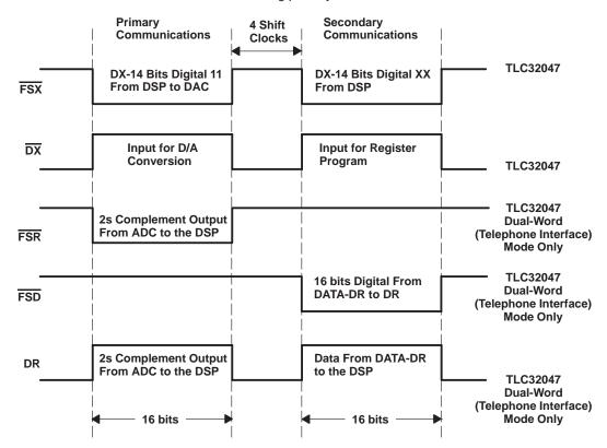
Figure 2-2. Primary and Secondary Communications Word Sequence
