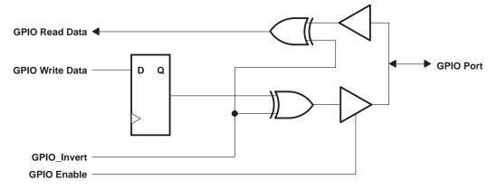
Figure 5–1. GPIO2 and GPIO3
