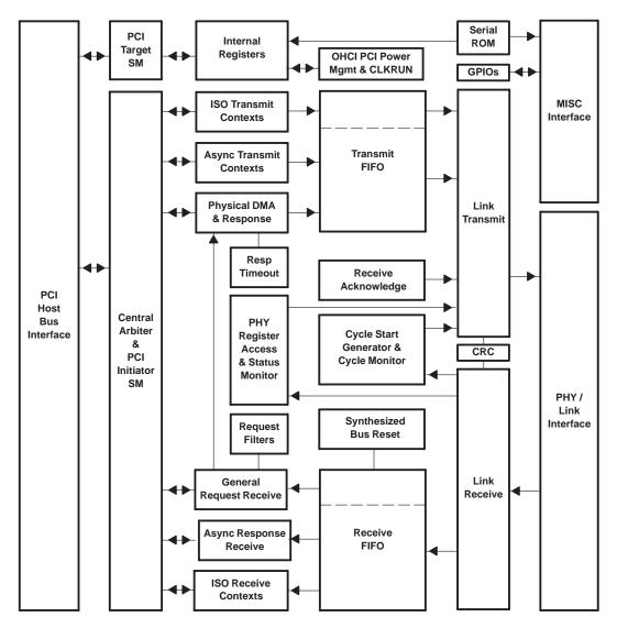
Figure 3–1. TSB12LV23 Block Diagram
