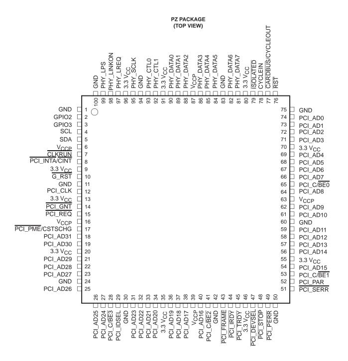
Figure 2–1. Terminal Assignments
