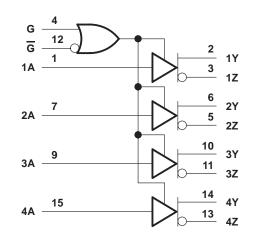
'LVDS9638 logic diagram (positive logic)
