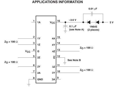
NOTE A: Place a 0.1 µF Z5U ceramic, mica or polystyrene dielectric, 0805 size, chip capacitor between V<sub>CC</sub> and the ground plane. The capacitor should be located as close as possible to the device terminals.
