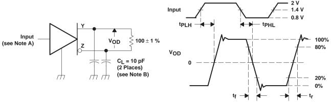
NOTES: A. All input pulses are supplied by a generator having the following characteristics:  $t_f \text{ or } t_f \le 1 \text{ ns}$ , pulse repetition rate (PRR) = 50 Mpps, pulse width = 10 ± 0.2 ns.
