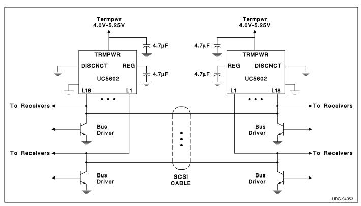
Typical SCSI Bus Configuration Using the UC5602
