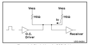
Figure 1. A Single Line of a SCSI Cable
