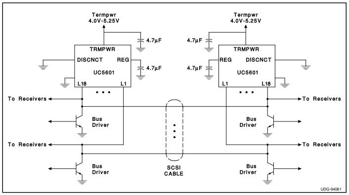
**Typical SCSI Bus Configuration Using the UC5601**
