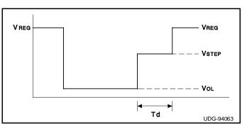
Figure 2. A Typical Response of a SCSI Cable
