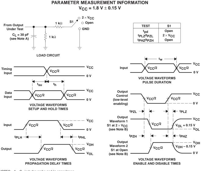
NOTES: A. CL includes probe and jig capacitance.
