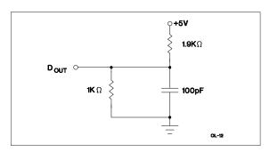
Figure 1. Output Load A
