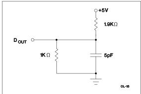
Figure 1. Output Load A
