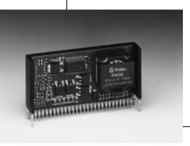
The PT7747 is a new high-performance 15 Amp "Current Booster" for the PT7750 Series housed in a 27-pin SIP package. Multiple PT7747 boosters will operate in parallel with the PT7750 Series boosting output current in increments of 15A. Combinations of PT7750s and PT7747 current boosters can easily supply enough power for virtually any multiple megaprocessor application.
