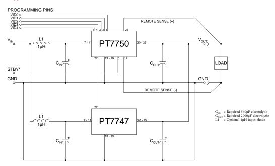
Output Capacitors: The PT7750/PT7747 series requires a minimum output capacitance of 2000µF for proper operation. Do not use Oscon type capacitors. The maximum allowable output capacitance is (42,000 4 Vout)µF for the PT7751, (96,000 4 Vout)µF for the PT7756, or 15,000µF, whichever is less.
