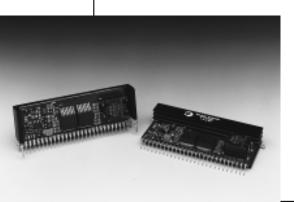
The PT7707 is a new series of high-performance, 18 Amp Integrated Switching Regulators (ISRs) housed in a 27-pin SIP package. The 18A capability allows easy integration of the latest high-speed, low-voltage µPs and bus drivers into existing 5V systems.
