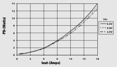
Note 1: All data listed in the above graphs has been developed from actual products tested at 25°C. This data is considered typical data for the ISR. Note 2: SOA curves represent operating conditions at which internal components are at or below manufacturer's maximum rated operating temperatures.
