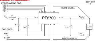
C<sub>in</sub> = Required 1000μF electrolytic Cout= Required 330µF electrolytic
