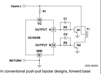
drive is controlled by R1-R3. Rapid turn-off times for the power devices are achieved with speed-up capacitors C, and C2.
