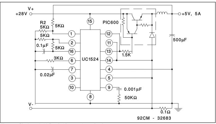
Figure 2. Single-ended LC switching regulator circuit.
