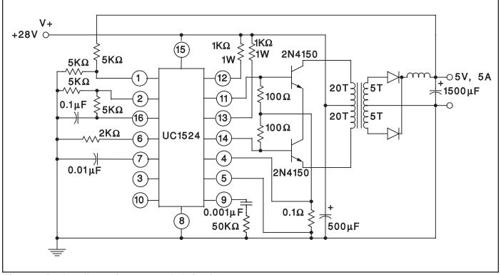
Figure 3. Push-pull transformer coupled circuit.
