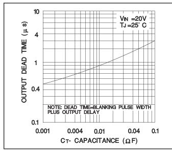
Output dead time vs timing capacitance value.
