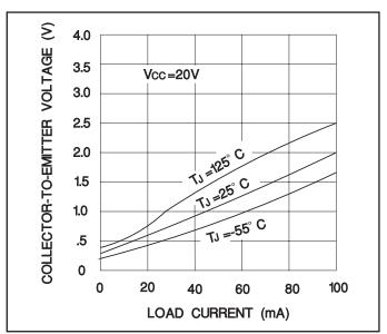
Output saturation voltage vs load current.
