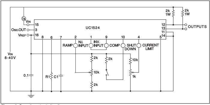
Figure 4. Open loop test circuit.
