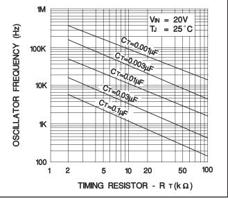
Oscillator frequency vs timing components.
