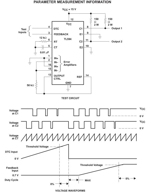
Figure 2. Operational Test Circuit and Waveforms
