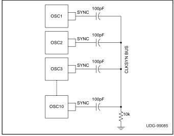
Figure 3. Oscillator synchronization connection diagram.
