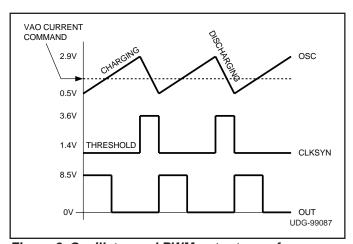
Figure 2. Oscillator and PWM output waveform.
