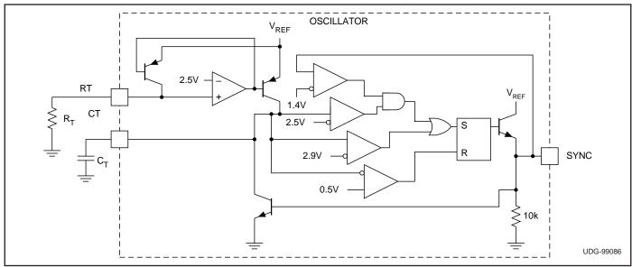
Figure 1. Oscillator block with external connections.
