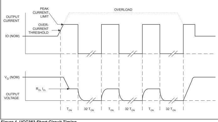
Figure 1. UCC383 Short Circuit Timing
