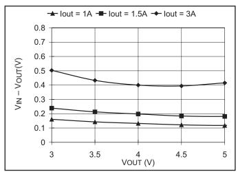
Figure 3. Typical Dropout Voltage vs. I<sub>OUT</sub> and V<sub>VOUT</sub>
