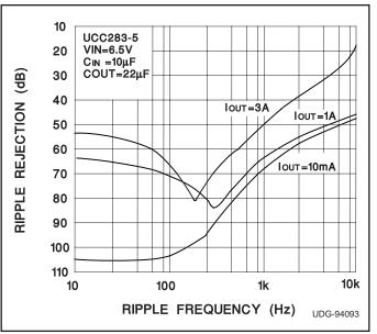
Figure 7. Ripple rejection vs. frequency.
