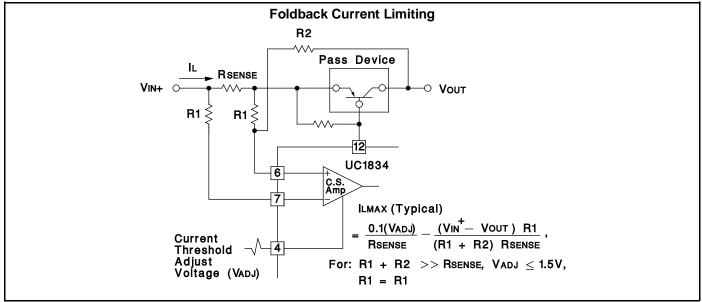
Both the current sense and error amplifiers on the UC1834 are transconductance type amplifiers. As a result, their voltage gain is a direct function of the load impedance at their shared output pin, Pin 14. Their small signal voltage gain as a function of load and frequency is nominally given by;
