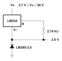
Figure 11. Operation Over a Wide Supply Range
