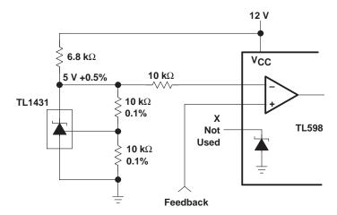
Figure 24. PWM Converter With 0.5% Reference
