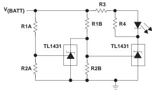
$$\begin{aligned} &\text{Low Limit} = \left(1 + \frac{R1B}{R2B}\right) V_{\text{I(ref)}} & & \\ &\text{High Limit} = \left(1 + \frac{R1A}{R2A}\right) V_{\text{I(ref)}} & & \\ &\text{Low Limit} < V_{\text{(BATT)}} < \text{High Limit} \end{aligned}$$
