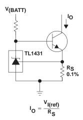
Figure 28. Precision Constant-Current Sink
