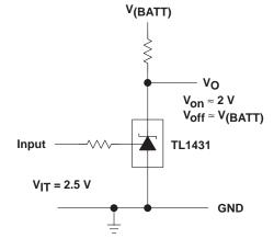
Figure 17. Single-Supply Comparator With Temperature-Compensated Threshold
