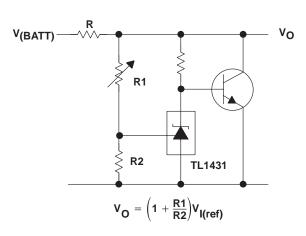
Figure 20. Higher-Current Shunt Regulator
