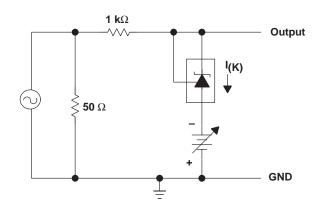
TEST CIRCUIT FOR REFERENCE IMPEDANCE
