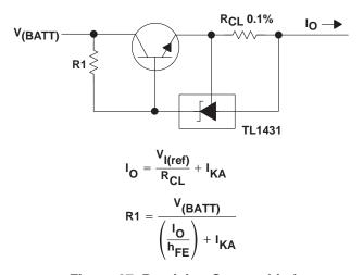
Figure 27. Precision Current Limiter
