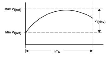
$\alpha_{V_{I(ref)}} \text{ is positive or negative depending on whether minimum } V_{I(ref)} \text{ or maximum } V_{I(ref)}, \text{ respectively, occurs at the lower temperature.}$
