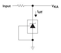
Figure 3. Test Circuit for I<sub>off</sub>
