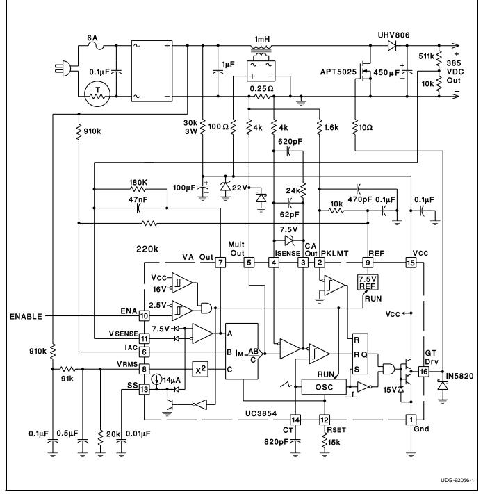
NOTE: Boost inductor can be fabricated with ARNOLD MPP toroidal core part number A-438381-2, using a 55 turn primary and a 13 turn secondary.
