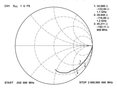
Figure 11. Typical RF\_IN Input Impedance (S<sub>11</sub>)
