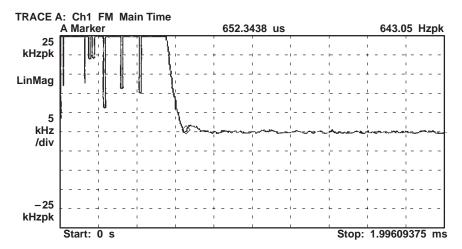
Figure 19. Typical Main Synthesizer Transient Response For 35-MHz Jump From 1074 MHz to 1109 MHz
