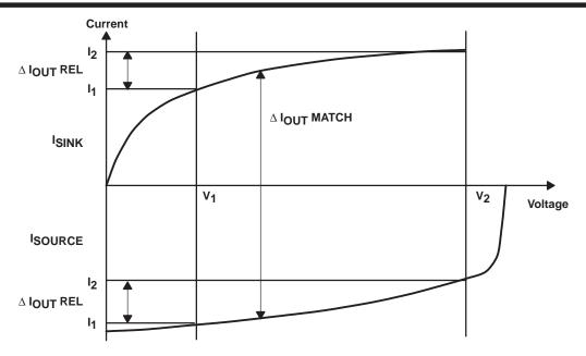
Figure 1. Charge-Pump Output Current Definitions
