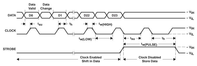
Figure 2. Serial Data Interface Timing
