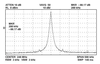
Figure 21. Typical Auxiliary-1 Synthesizer Reference Spurs
