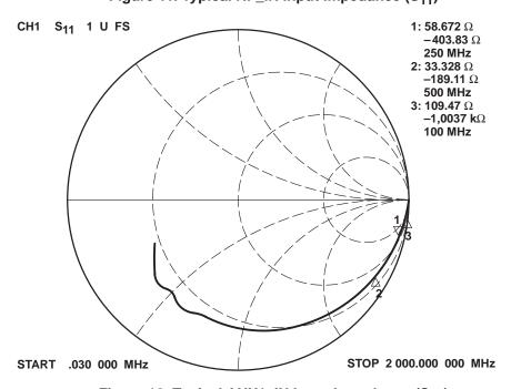
Figure 12. Typical AUX1\_IN Input Impedance (S<sub>11</sub>)
