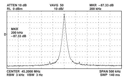
Figure 22. Typical Auxiliary-2 Synthesizer Reference Spurs
