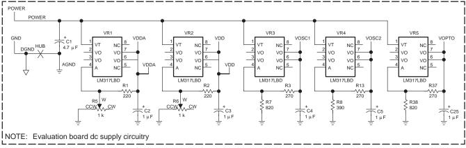
Figure 15. Evaluation Board Schematic (Part 2 of 2)
