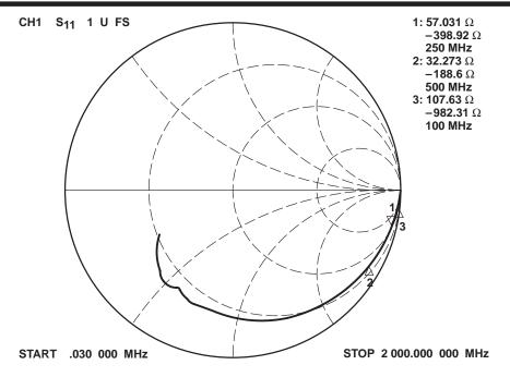
Figure 13. Typical AUX2\_IN Input Impedance (S<sub>11</sub>)
