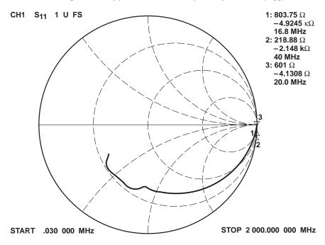
Figure 14. Typical REF\_IN Input Impedance (S<sub>11</sub>)
