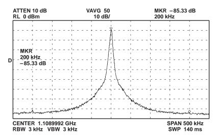
Figure 16. Typical Main Synthesizer Reference Spurs
