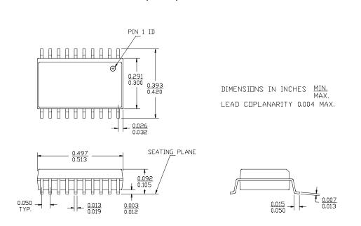
20-Lead (300-Mil) Molded SOIC S5
