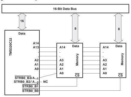
Figure 3. 'C32 With 16-Bit-Wide External Memory
