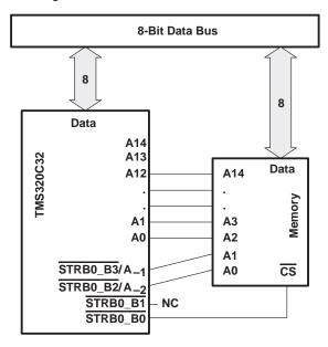
Figure 2. 'C32 With 8-Bit-Wide External Memory
