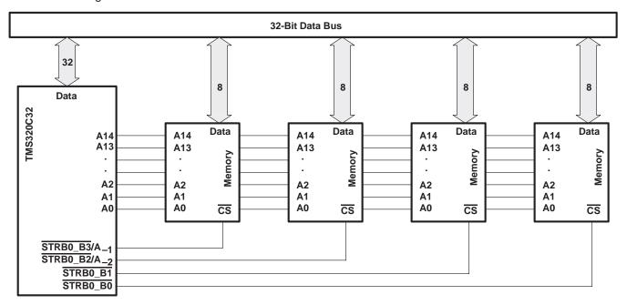
Figure 4. 'C32 With 32-Bit-Wide External Memory
