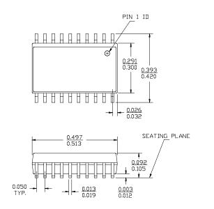
DIMENSIONS IN INCHES MIN. LEAD COPLANARITY 0.004 MAX.
