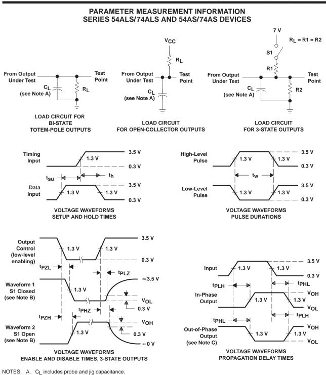
B. Waveform 1 is for an output with internal conditions such that the output is low except when disabled by the output control. Waveform 2 is for an output with internal conditions such that the output is high except when disabled by the output control.
