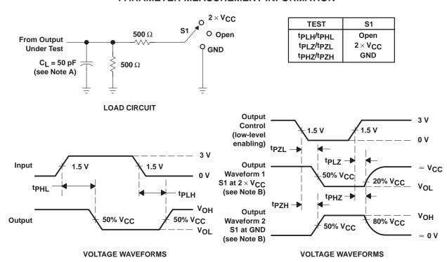
NOTES: A. C<sub>I</sub> includes probe and jig capacitance.
