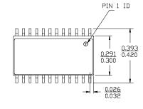
DIMENSIONS IN INCHES  $\frac{\text{MIN.}}{\text{MAX.}}$  LEAD COPLANARITY 0.004 MAX.
