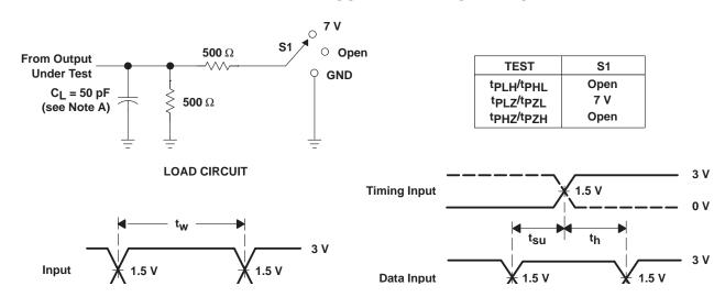
Figure 1. Load Circuit and Voltage Waveforms
