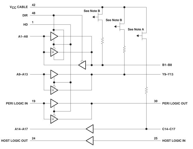
NOTES: A. The PMOS prevents backdriving current from the signal pins to V<sub>CC</sub> CABLE when V<sub>CC</sub> CABLE is open or at GND.
