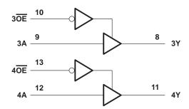
Pin numbers shown are for the D, DB, DGV, J, NS, PW, and W packages.
