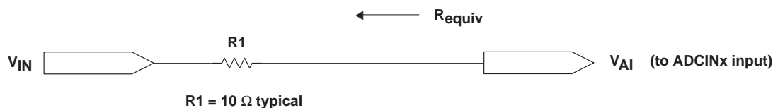
Figure 42. Typical ADC Input Pin Circuit
