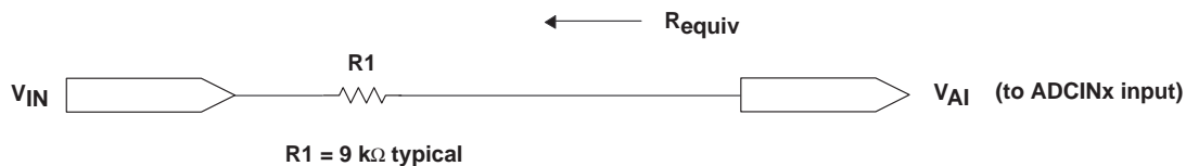
Figure 46. Typical ADC Input Pin Circuit
