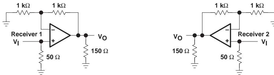
Figure 2. Receiver Input-to-Output Crosstalk Test Circuit
