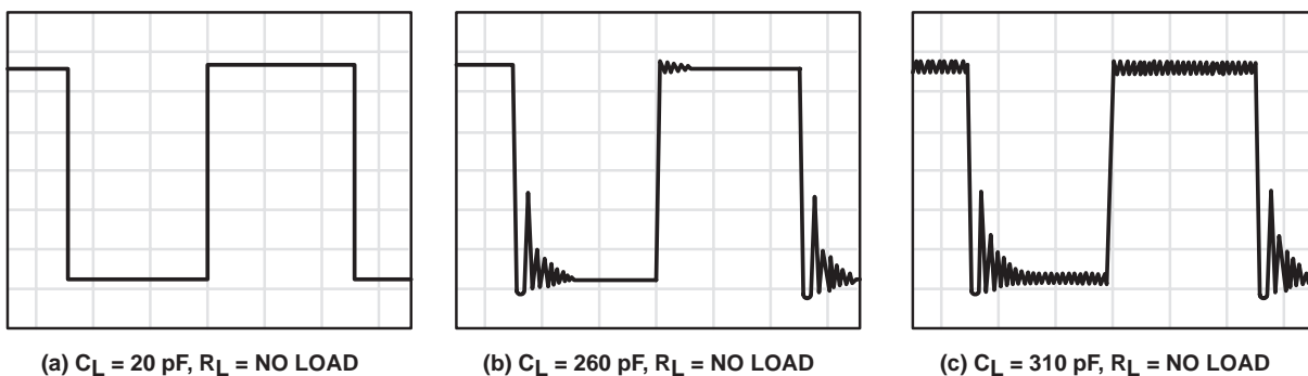
Figure 44. Effect of Capacitive Loads in Low-Bias Mode
