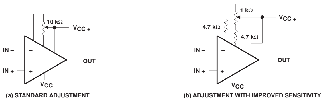
Figure 55. Input Offset Voltage Nulling Circuits
