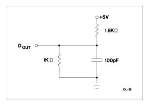
Figure 4. Output Load A
