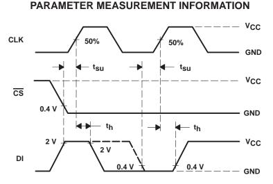
Figure 1. Data-Input Timing
