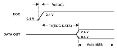
Figure 7. Data Output to EOC Timing
