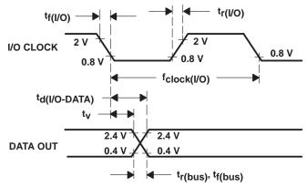
Figure 5. Data Output Timing
