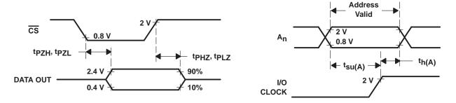
Figure 2. CS to Data Output Timing
