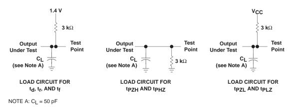
Figure 1. Load Circuits
