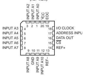
analog multiplexer can sample any one of 11 inputs or an internal "self-test" voltage, and the sample and hold is started under microprocessor control. At the end of conversion, the end-of-conversion (EOC) output pin goes high to indicate that conversion is complete. Detailed information on interfacing to most popular microprocessors is readily available from the factory.
