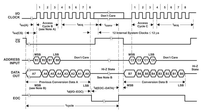
NOTES: A. To minimize errors caused by noise at the chip select input, the internal circuitry waits for two rising edges and one falling edge of the internal system clock after CS↓ before responding to control input signals. The CS setup time is given by the t<sub>Su(CS)</sub> specifications. Therefore, no attempt should be made to clock-in an address until the minimum chip select setup time has elapsed.
