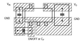
Use a large bypass capacitor and connect it in a place near GND of the IC. Pay attention to temperature characteristics of the capacitor, especially the increase of ESR and decrease of capacitance in low temperatures. Oscillation, reduction of ripple rejection and increased noise may occur in some cases if the proper capacitor is not used. An output capacitor more than 1.0  $\mu$ F is required to maintain stability. The standard test condition is 3.3  $\mu$ F (T<sub>A</sub> = 25 °C).
