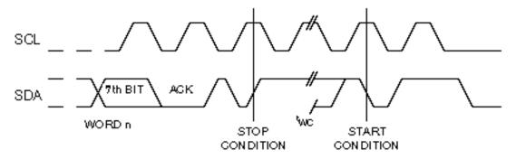
Note: The write cycle time  $t_{\text{WC}}$  is the time from a valid stop condition of a write sequence to the end of the internal clear / write cycle.
