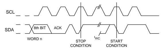
Note: The write cycle time  $t_{\text{WC}}$  is the time from a valid stop condition of a write sequence to the end of the internal clear / write cycle.
