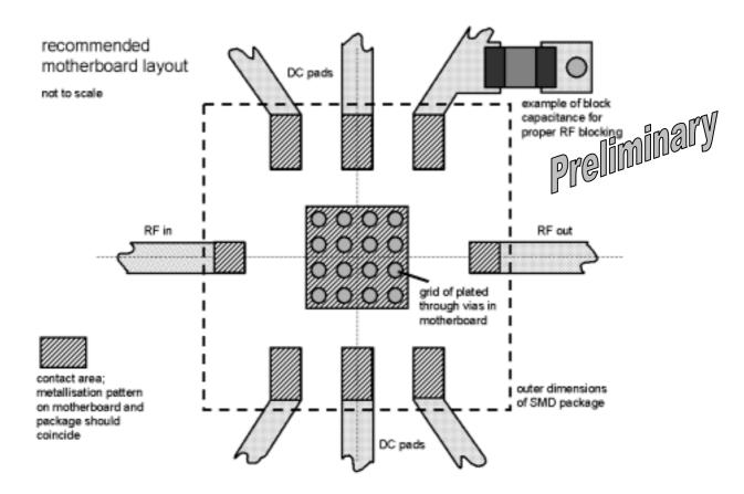
The RF ports comprise a DC blocking capacitor on chip level. The DC connections include a first level of DC decoupling capacitors (typically 120pF) in the package. However, all DC bias ports should be additionally connected to ground with 10nF capacitors at board level to prevent the MMIC from oscillations. These parts should be placed close to the SMD leadless package. If the same bias is required at different DC ports, the lines should only be connected behind these block capacitors.
