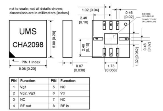
"Please note that PIN 1 is located in the lower left corner of the package (front-side view) for all SMD-type packages from United Monolithic Semiconductors. It is indicated by a triangle on the package lid. Starting with PIN 1 the other pads are numbered counter-clockwise (front-side view). ATTENTION: The dot on the backside of the package (i.e. side with metallic pads) is just for fabrication purposes and does NOT indicate the location of PIN
