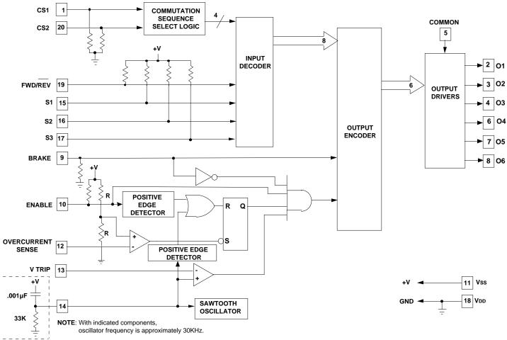
FIGURE 6. LS7260 AND LS7262 BLOCK DIAGRAM
