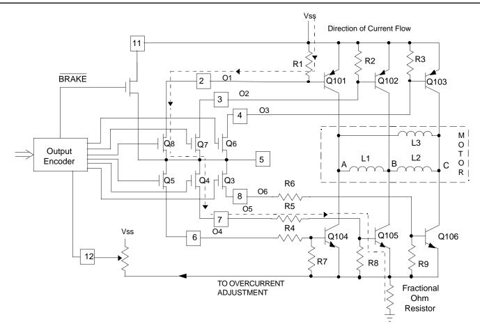
FIGURE 2. LS7262 THREE PHASE OUTPUT DRIVER CIRCUITRY
